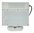
PN Canceller is not just a conventional repeater such as RF or ICS repeater but a smart repeater system with identifying the cells and analyzing the link quality between node-Bs and service area. PN Canceller can convey only the good signal by cancellation the other bad signals which invokes the unnecessary network resources such as channel card, radio link in RNC etc,. It includes interference cancellation function as well to suppress the feedback signal.
